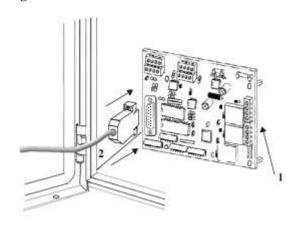
The Version 9.1 PCB are configured so that this connector is positioned vertically along the inner side of the enclosure.
