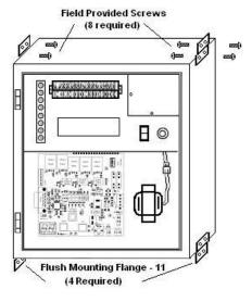
For best Flush Mounting results, recess face of enclosure's lip 1/4" behind wall finish
