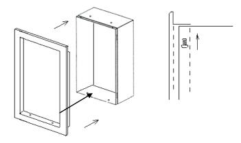
If the Controller HUB is flush mounted, a Trim Kit is provided.
